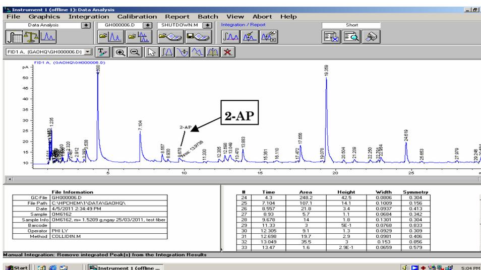
Fig 6. SPME/GC-FID chromatograph of OM 6162 exposed the peak 2-AP at the Rt 9.678 minute
