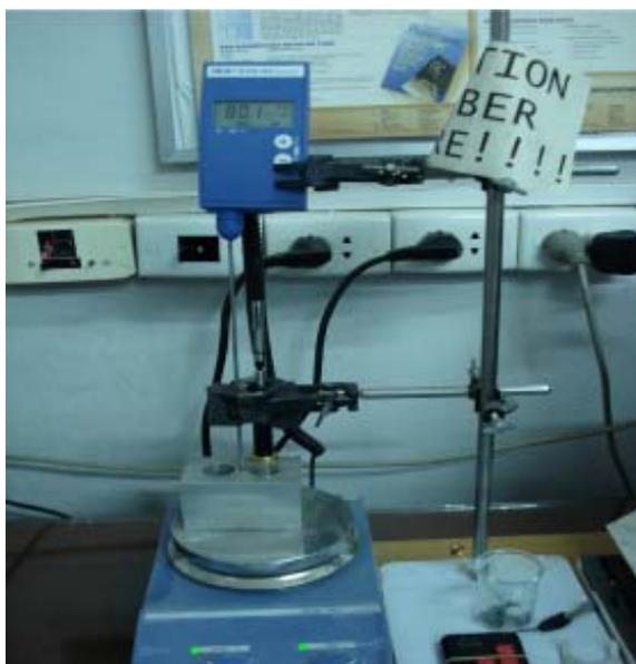
**Fig 2. System of the SPME extraction**
