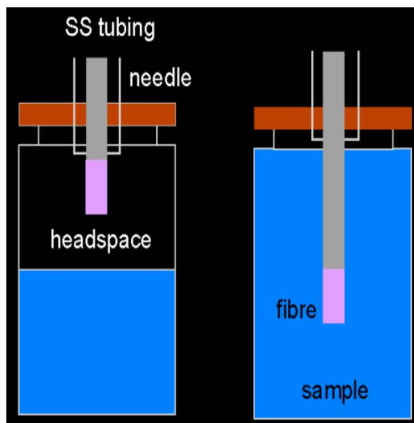
**Fig 3. Adsorption phase in SPME extraction**
