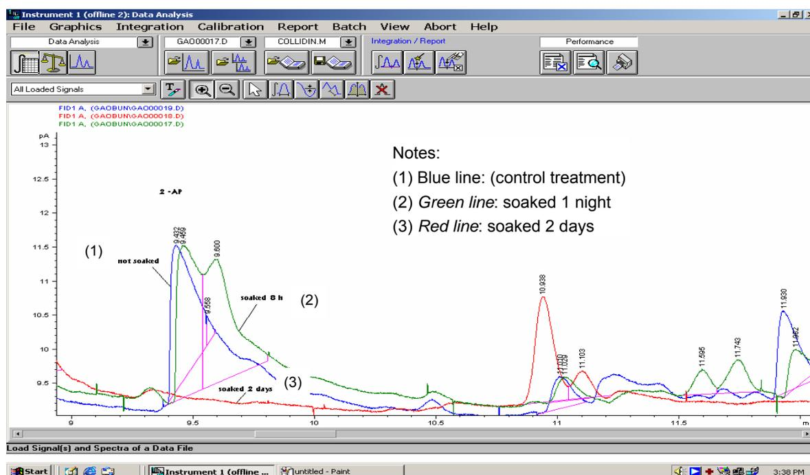
**Fig 7. GC-FID chromatograph found out the change of 2-AP and other volatile compounds in three treatments: KDM not to be soaked, to be soaked for 8 hours, and for 2 days.**
