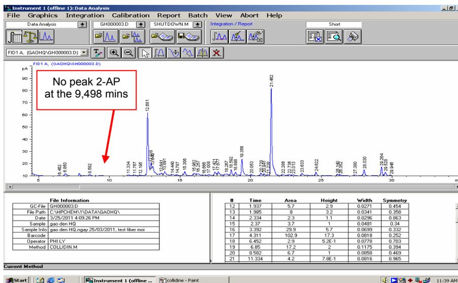
Fig 5. Volatile compounds in Chucheong rice from Korea recorded by GC-FID showed that it has no peak 2-AP at the Rt 9.498 minute
